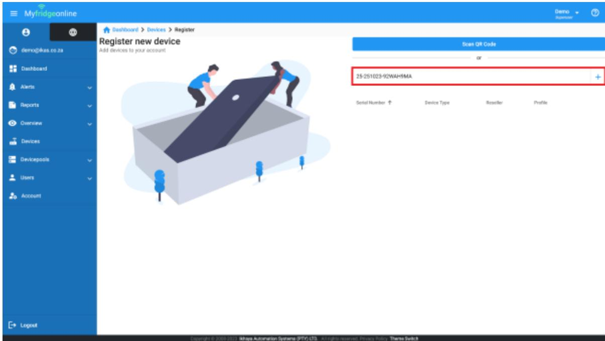
5. The serial number will then be entered into the table. Step 4 can be repeated if multiple devices are to be registered. Once complete click 'Register Devices' to complete registering devices to your account and your devices will then be displayed on the Devices page.
