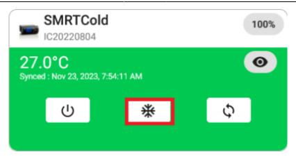
Clicking on the continuous cycle button will set the unit to continuous cycle. This will also be visually indicated on the device by the same icon.
